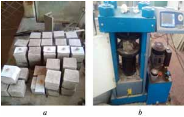
Fig. 2. The experimental concrete samples (a) and the process of crushing an experimental concrete sample (b) under an hydraulic press in the laboratory
