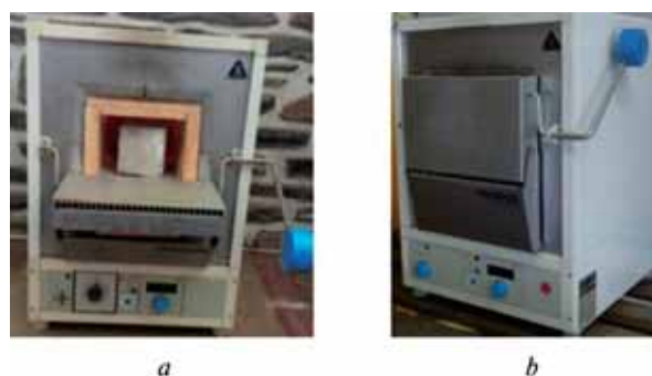
Fig. 2. Electrical furnace with experimental sample with the door open (a) and the electrical furnace with the closed-door (b)
