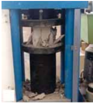
Fig. 3. Compression test on heated experimental samples
