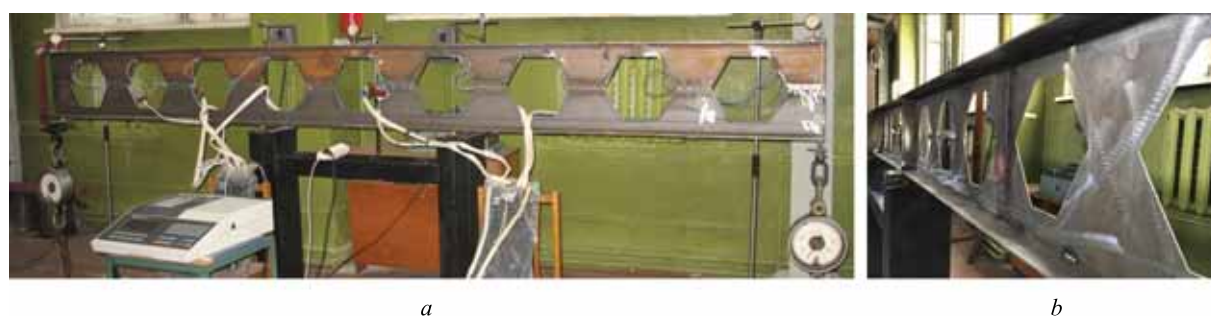
Fig. 16. Testing set up for determination of beam's deflections: a — with wide web-posts \xi = 1 ; b — with narrow web-posts \xi = 0.4
